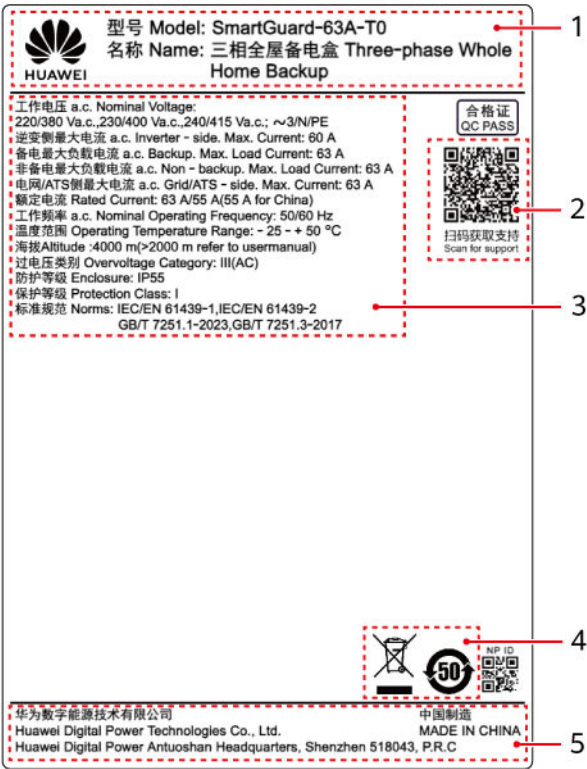
Figure 2-13 Nameplate (SmartGuard-63A-T0 as an example)
